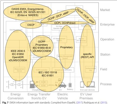
**Fig. 7** EMSA information layer with standards. Compiled from ElaadNL (2017); Rodríguez et al. (2015); Schmutzler et al. (2013)
